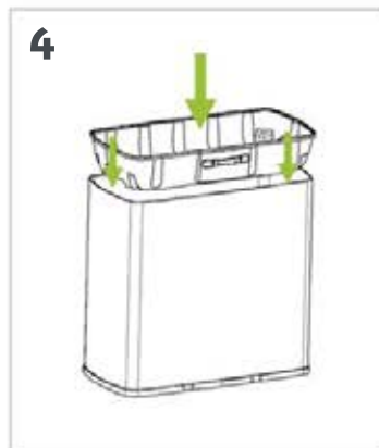
4 Positionner la partie vide du container en haut de la jupe pour rigidifier la structure. Place the bottom lid, rounded portion facing down into the top of the roll. This will tighten the roll form the structure and maintain stability.
